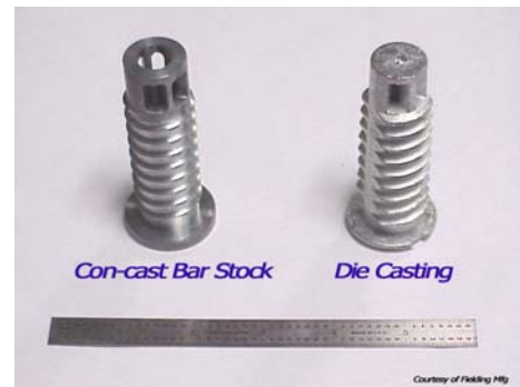
Figure 3 – Inject Solutions Plug. Con-cast bar stock (left), Die Casting (right).
