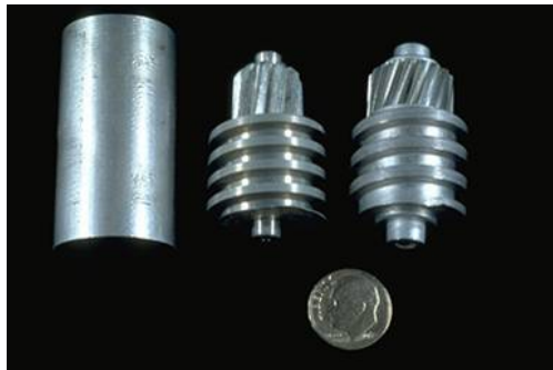
Figure 4 - Male Drive Spline for A Power Seat Drive Assembly
